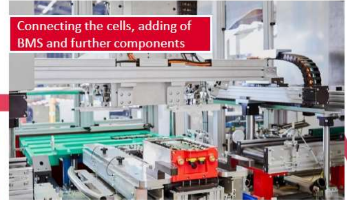
Assembling of produced modules to systems
